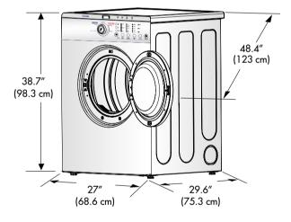
\* Most installations require a minimum 5 1/2 in. (14 cm) clearance behind the dryer for the exhaust vent with elbow.
